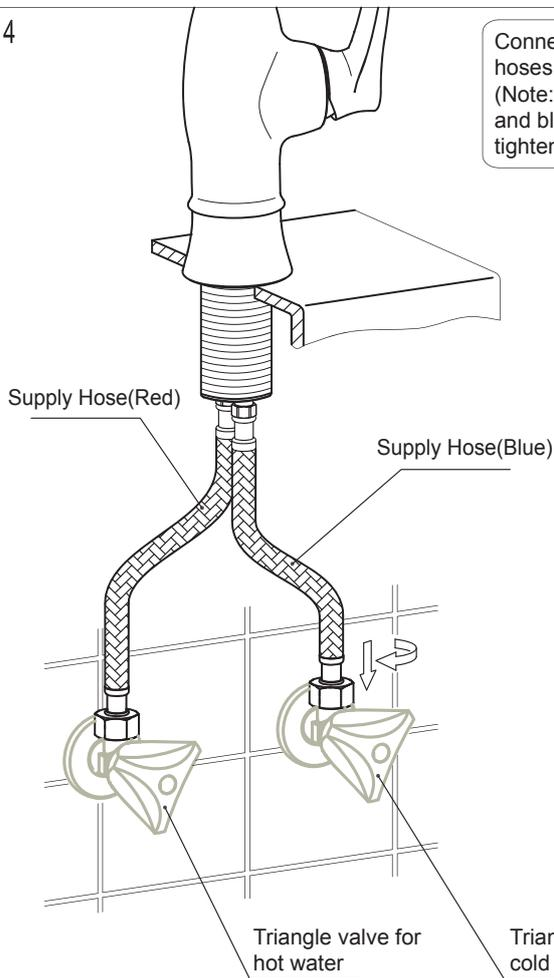
Connect two supply hoses to triangle valves (Note: red for hot water and blue for cold water), tighten with spanner.
