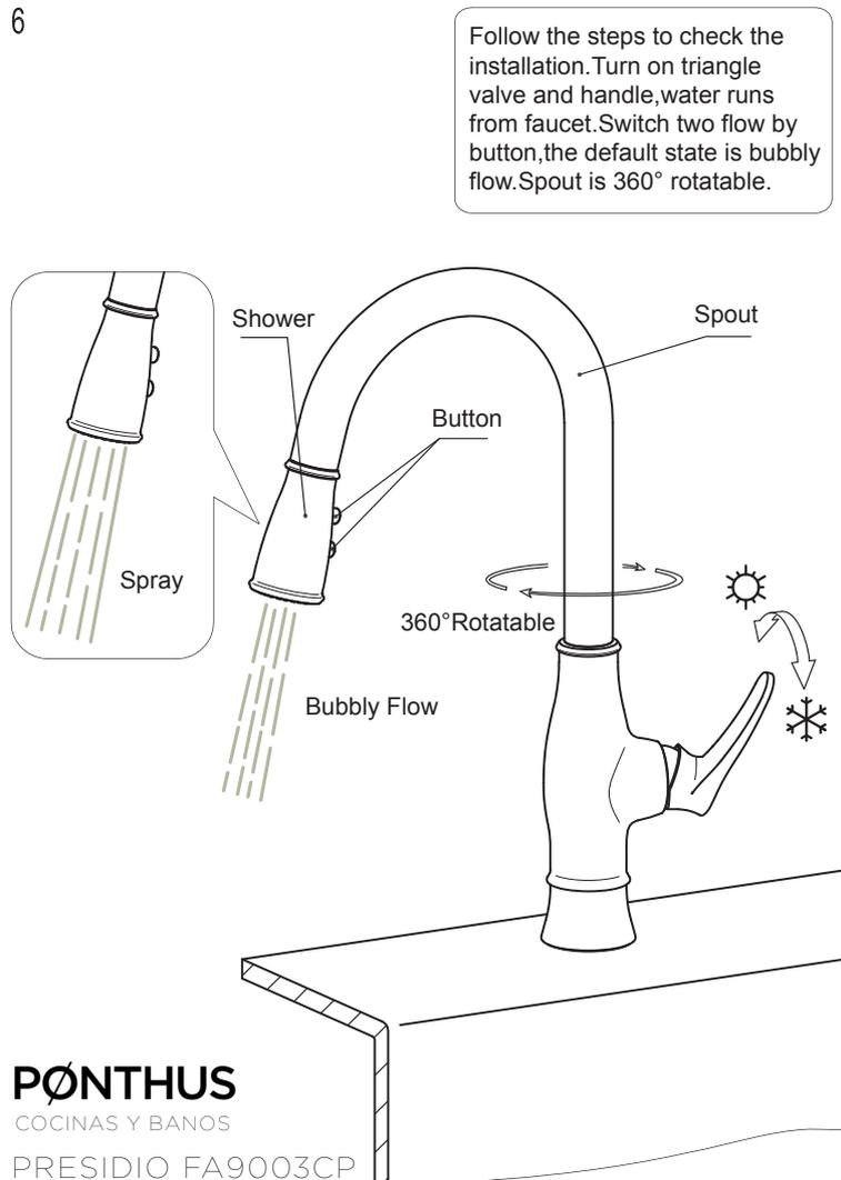
Follow the steps to check the installation. Turn on triangle valve and handle, water runs from faucet. Switch two flow by button, the default state is bubbly flow. Spout is 360° rotatable.
