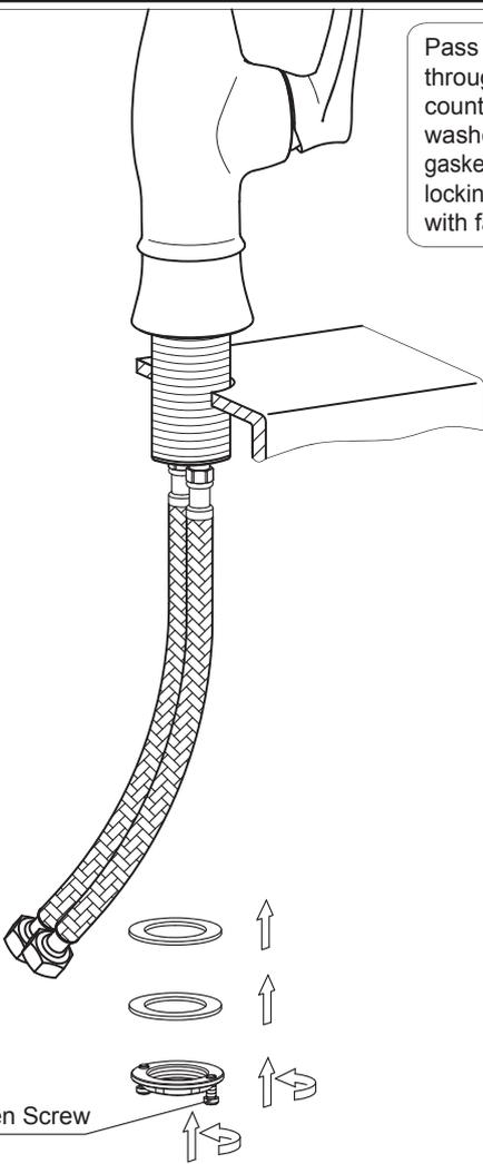
Pass faucet body through hole of sink counter, pad rubber washer and locking gasket in turn, screw on locking nuts and secure with fasten screw.
